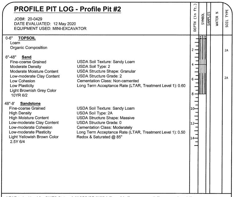
LTAR to be Used for OWTS Sizing: 0.50GPD/SF (USDA Type 2A, Treatment soil, Treatment Level 1)
