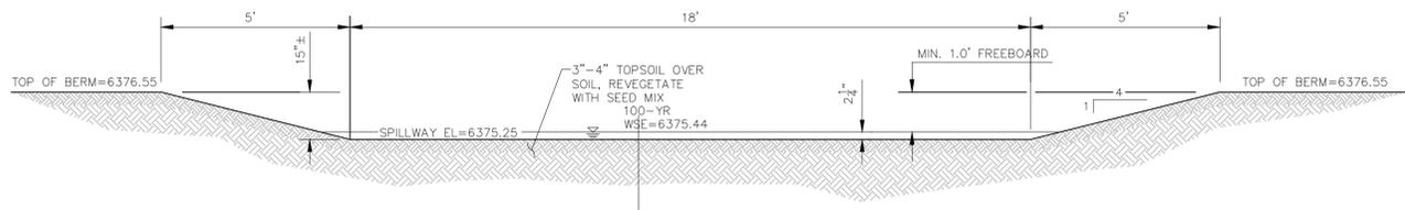
**SPILLWAY CREST SECTION A-A**
