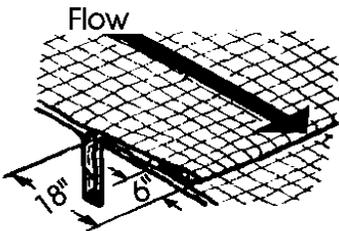
**Joining Strips:** Insert the new roll of net in a trench, as with the Anchor Slot. Overlap the up-channel end of the previous roll 18" and turn the end under 6". Staple the end of the previous roll just below the anchor slot and at the end at 12" intervals.
