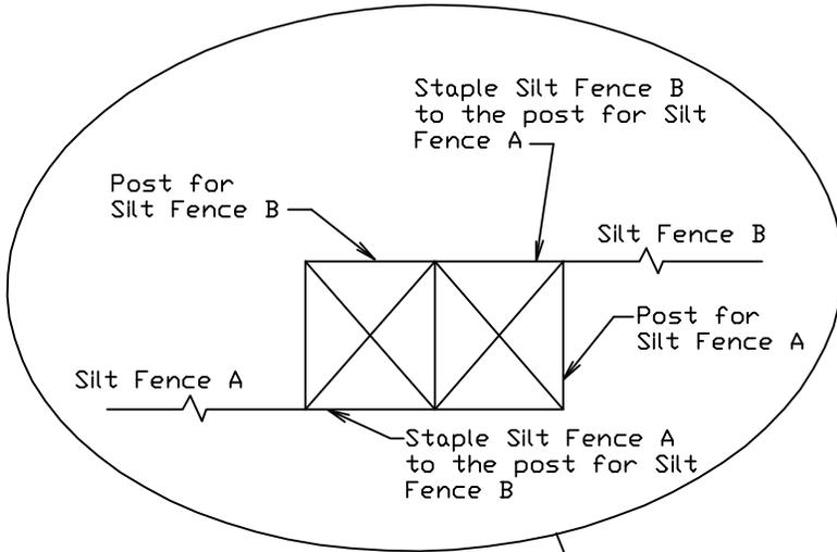
Refer to "Top View of Silt Fence Posts Detail"
