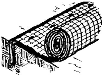
**Anchor Slot:** Bury the up-channel end of the net in a 6" deep trench. Tamp the soil firmly. Staple at 12" intervals across the net.
