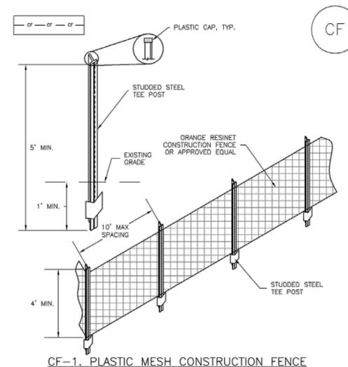
**CF-1. PLASTIC MESH CONSTRUCTION FENCE**
