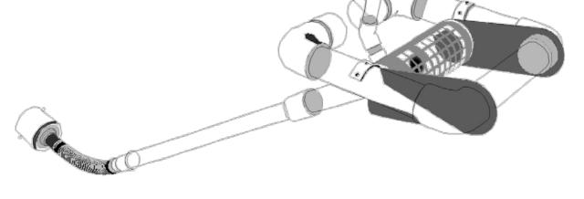
Illustration SB-1. Outlet structure for a temporary sediment basin - Faircloth Skimmer Floating Outlet. Illustration courtesy of J. W. Faircloth & Sons, Inc., FairclothSkimmer.com.
