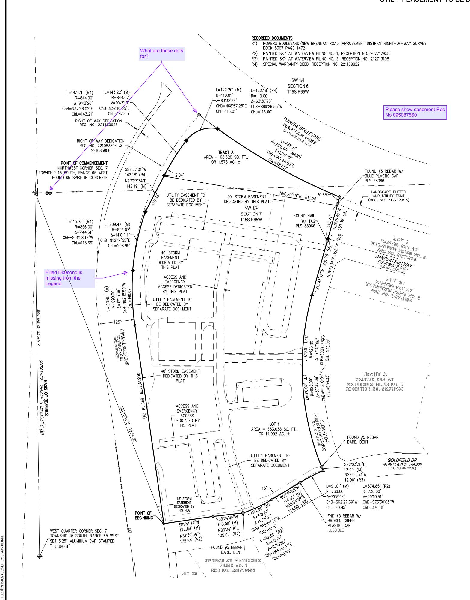
LEGEND FOUND MONUMENT AS DESCRIBED ♦ FOUND #5 REBAR W/ GREEN PLASTIC CAP, PLS 38245 △ FOUND #5 REBAR W/ YELLOW PLASTIC CAP, PLS 34583 SET #5 REBAR W/ RED PLASTIC CAP OR TAG, WHERE APPLICABLE PLS 38061 ◆ PLSS SECTION CORNER (M) MEASURED VALUES (R) RECORDED VALUES SURVEYED PROPERTY BOUNDARY - - EXISTING RIGHT-OF-WAY LINE RIGHT-OF-WAY DEDICATED BY THIS PLAT ACCESS EASEMENT DEDICATED BY THIS PLAT STORM DRAIN EASEMENT DEDICATED BY THIS PLAT UTILITY EASEMENT TO BE DEDICATED BY SEPARATE DOCUMENT
