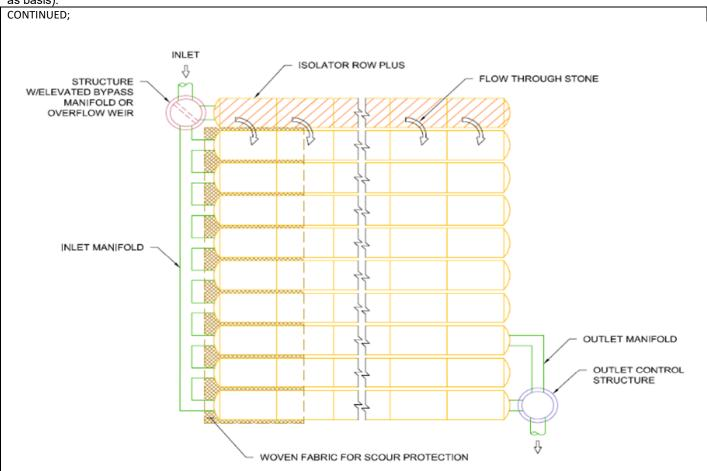
THE XK BAYSEPARATOR IS LOCATED SIMILAR TO THE "STRUCTURE W/ELEVATED BYPASS MANIFOLD OR OVERFLOW WEIR" SHOW IN THE DETAIL ABOVE AT THE INLET SIDE OF THE SYSTEM. THE ISOLATOR ROWS ARE ALSO ON THE INLET SIDE OF THE SYSTYEM AFTER THE XK BAYSEPARATOR.
