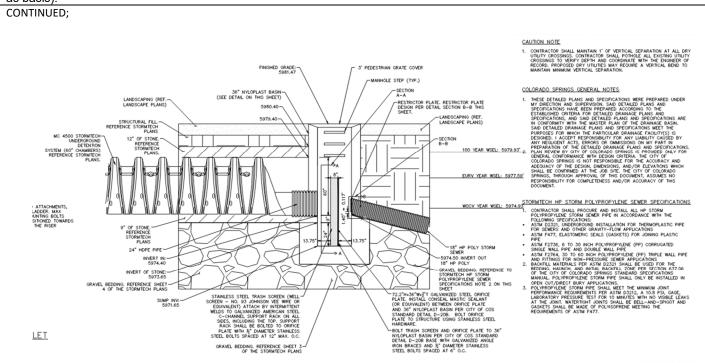
SIMILAR TO AN ABOVE GROUND POND DESIGN, THE OVERALL DRAIN TIME AND RELEASE RATES WILL BE CONTROLLED WITHIN THE OUTLET STRUCTURE. A STAGE AREA SPREADSHEET WILL BE USED TO INCORPORATE THE DATA INTO THE MHFD DETENTION SPREADSHEET FOR OUTLET STRUCTURE SIZING.
