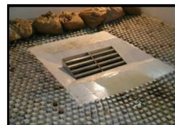
CDOT Type D Inlet Parallel (20° Incline & Depressed)
