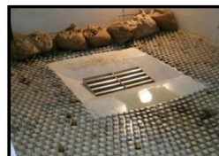
CDOT Type D Inlet Parallel (10° Incline & Depressed)
