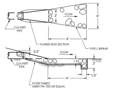
**RIPRAP AT DRAIN PIPE ENDS**
