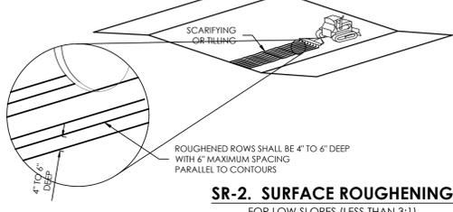
**SR-2. SURFACE ROUGHENING FOR LOW SLOPES (LESS THAN 3:1)**
