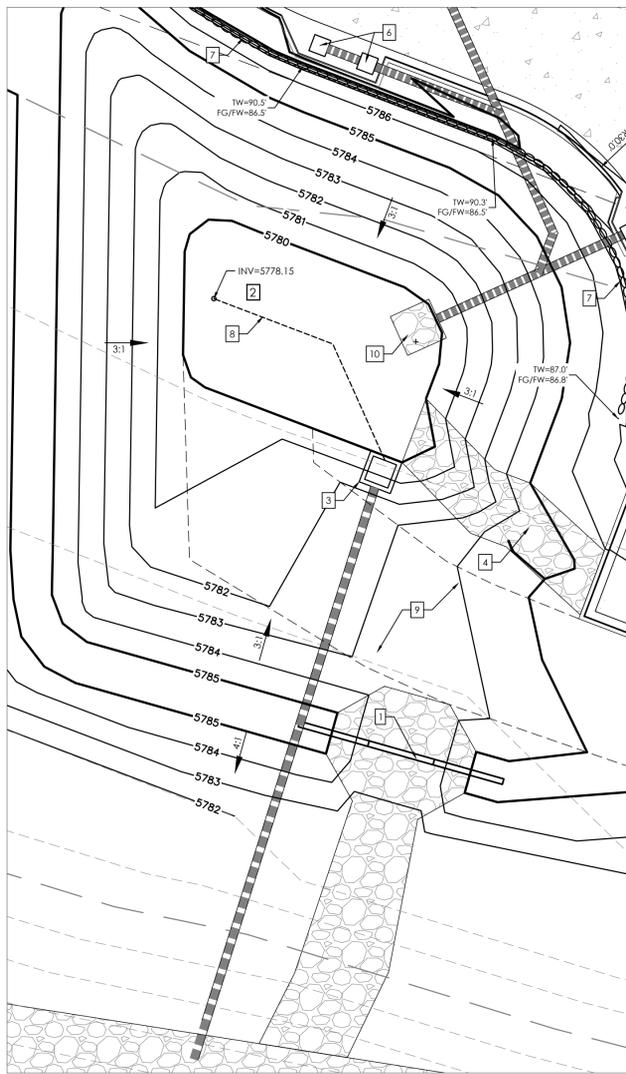
**EXTENDED DETENTION SAND FILTER BASIN DETAIL**
