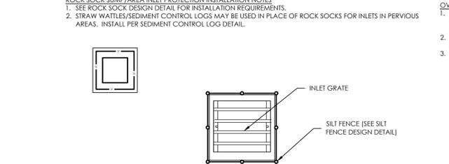
**IP-4. SILT FENCE FOR SUMP INLET PROTECTION**
