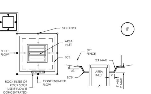
**IP-5. OVEREXCAVATION INLET PROTECTION**
