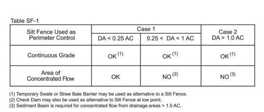
Figure SF-1 City of Colorado Springs Silt Fence Storm Water Quality
