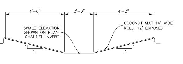
**DRAINAGE DITCH (DD1)** SCALE 1"=2'-0"
