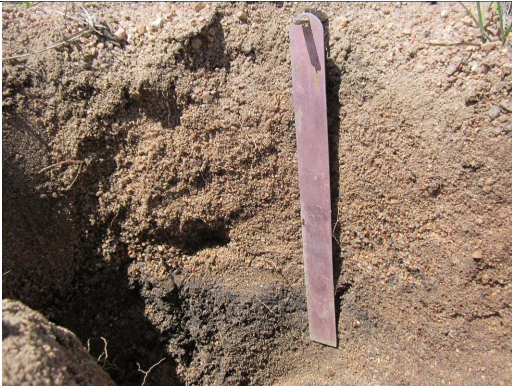
Photo 7: Soil profile at OHWM datasheet showing recent sandy erosional deposit
