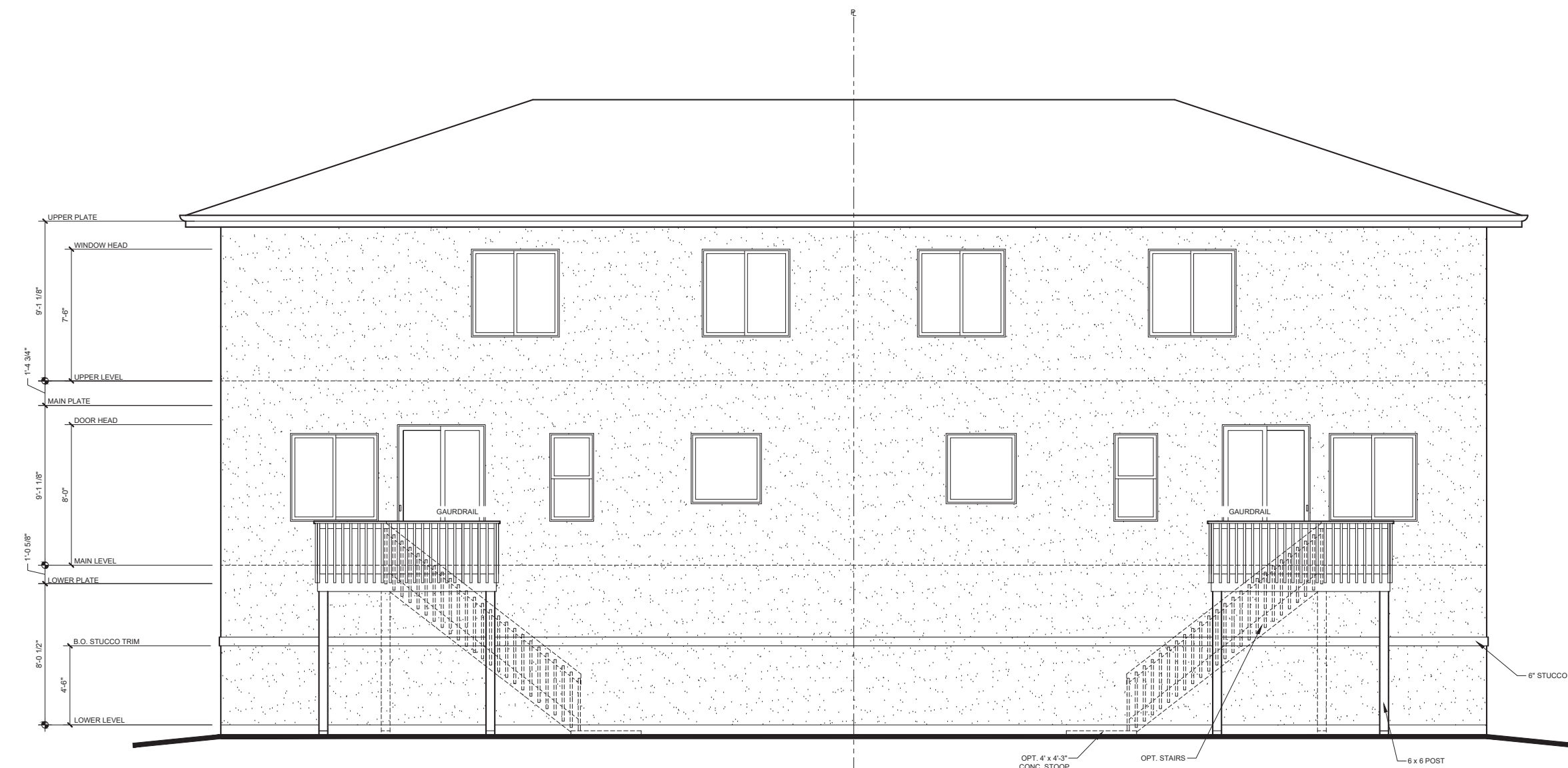
1 OPT. WALKOUT REAR ELEVATION - 'C' SCALE: 1/4" = 1'-0"
