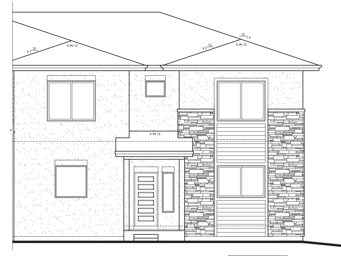
2 OPT. FRONT ELEVATION - 'C' SCALE: 1/4" = 1'-0"
