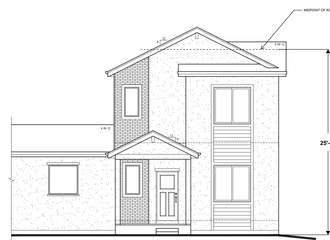
② OPT. FRONT ELEVATION - 'B' SCALE: 1/4" = 1'-0"
