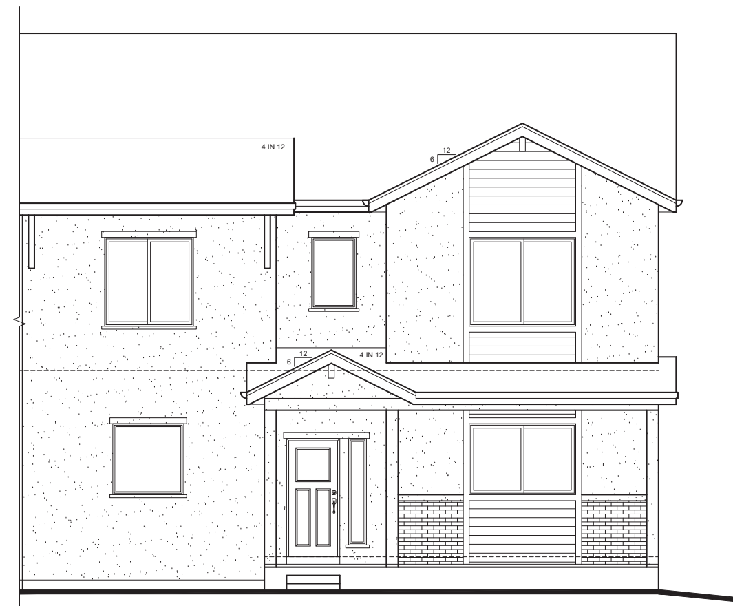
2 OPT. FRONT ELEVATION - 'B' OPT. ALLEY LOAD GARAGE SCALE: 1/4" = 1'-0"
