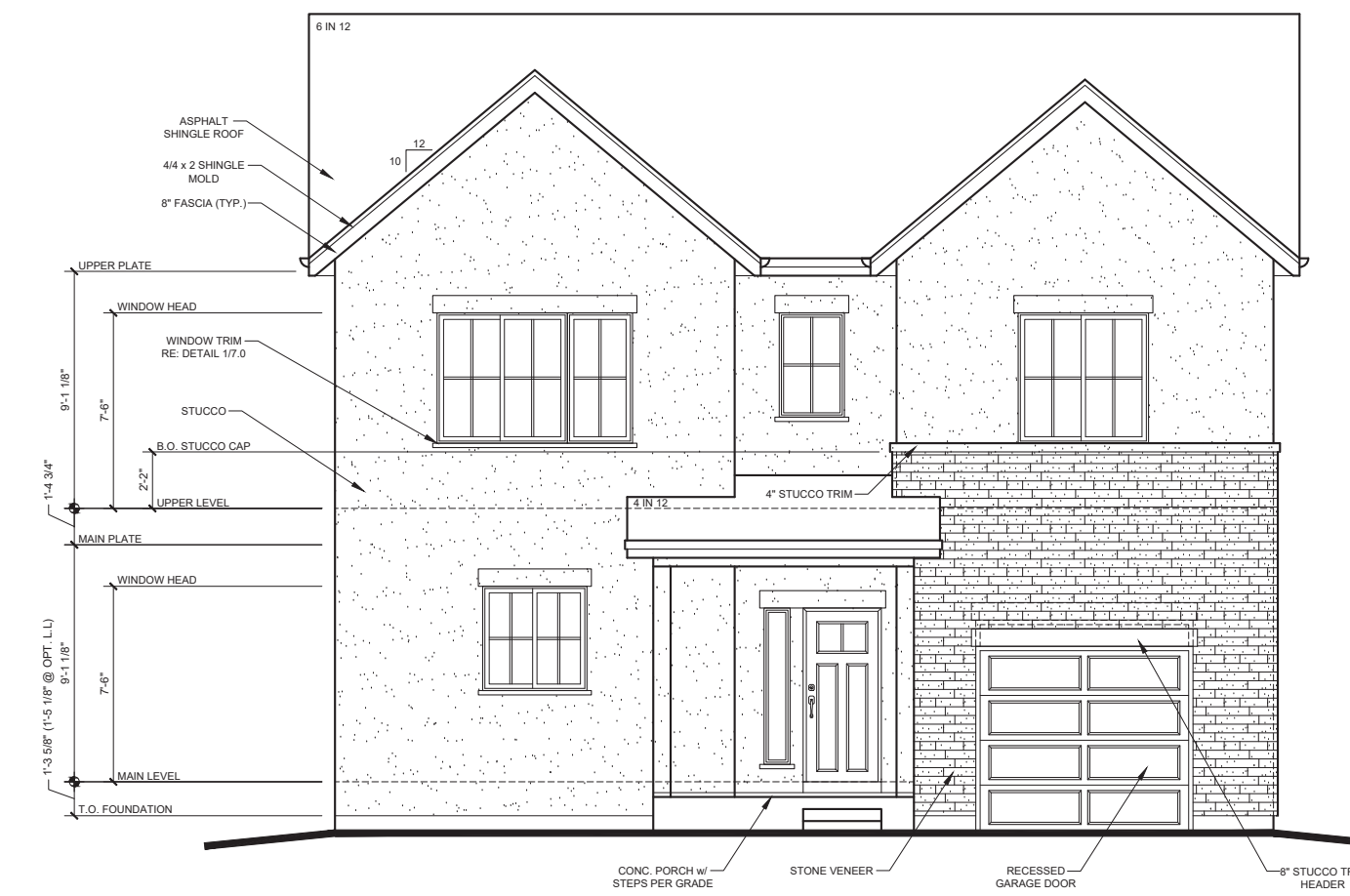
1 FRONT ELEVATION - 'A' SCALE: 1/4" = 1'-0"
