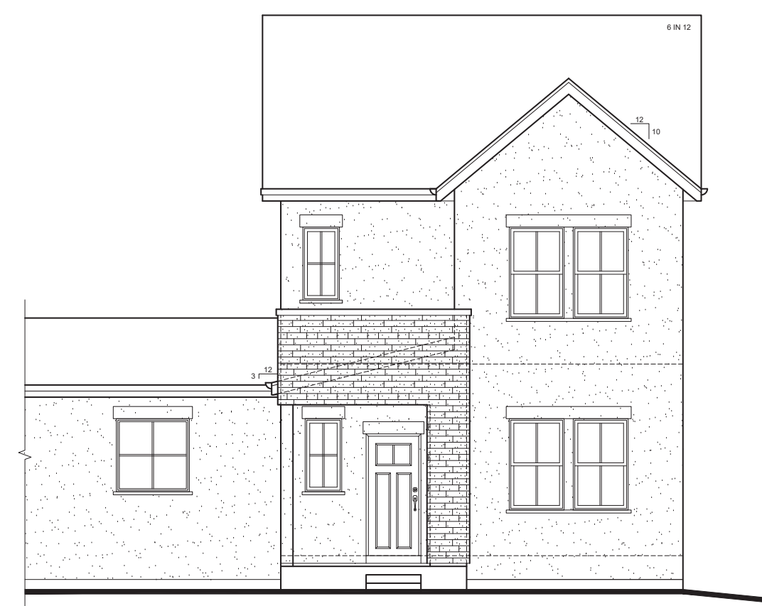
2 OPT. FRONT ELEVATION - 'A' SCALE: 1/4" = 1'-0" OPT ALLEY LOAD GARAGE
