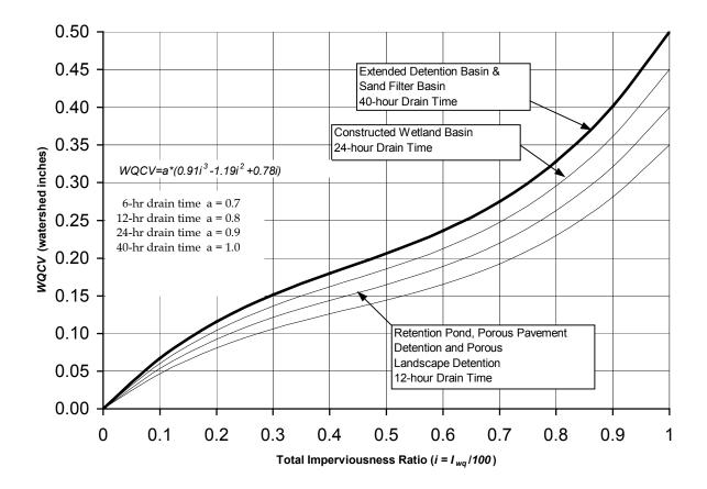
FIGURE SFB-2 Water Quality Capture Volume (WQCV), 80<sup>th</sup> Percentile Runoff Event
