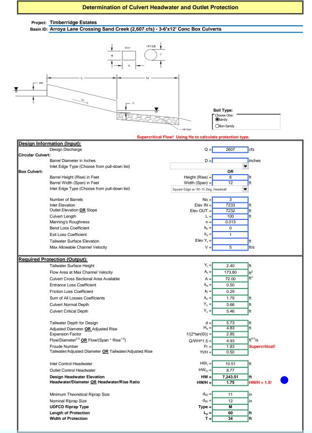
The south report provided an analysis of 3-6x16 RCBCs. Discuss options, including what size would be required to meet the 2-foot freeboard requirement (entering the culvert).
