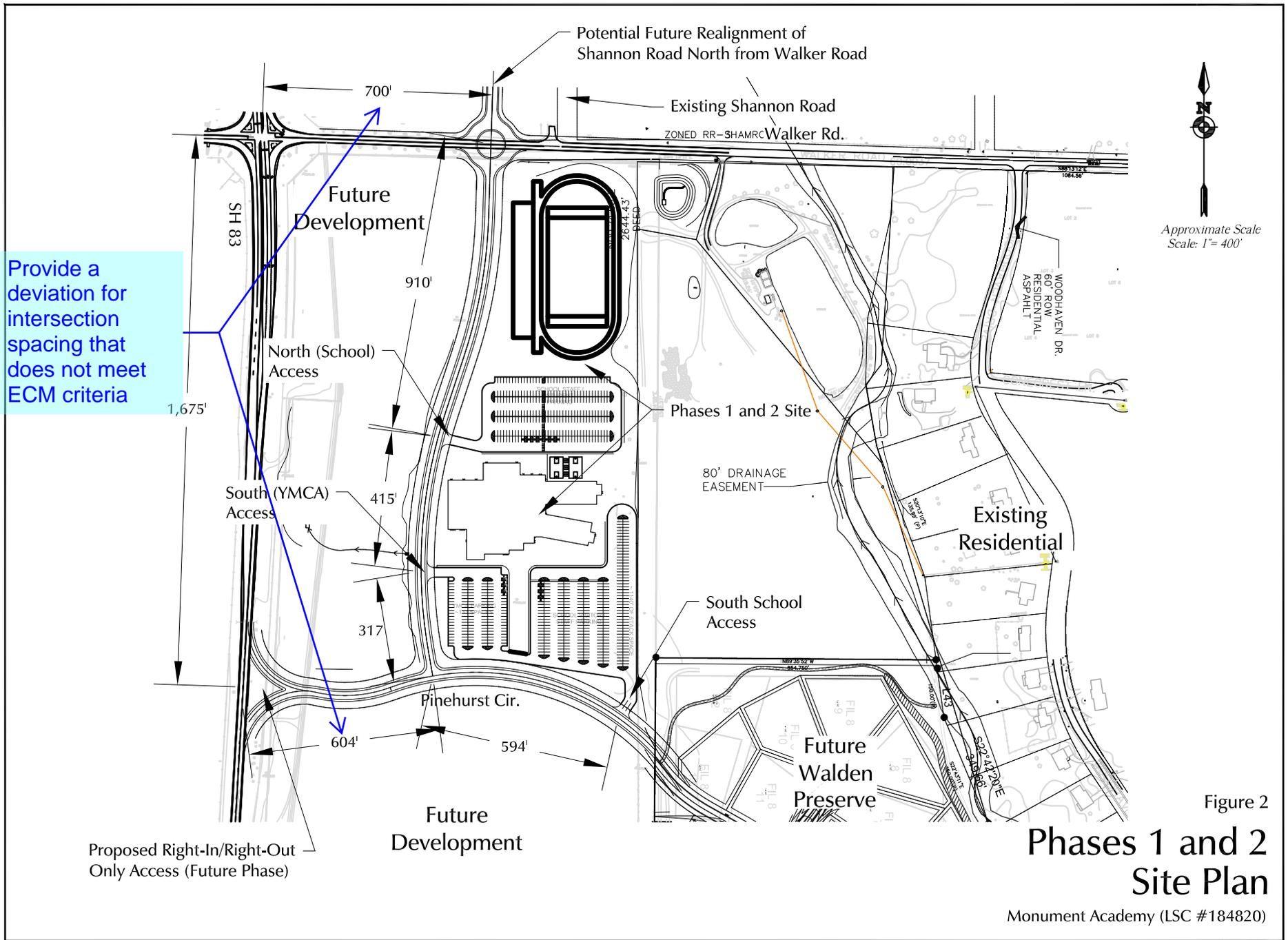
Provide a deviation for intersection spacing that does not meet ECM criteria
