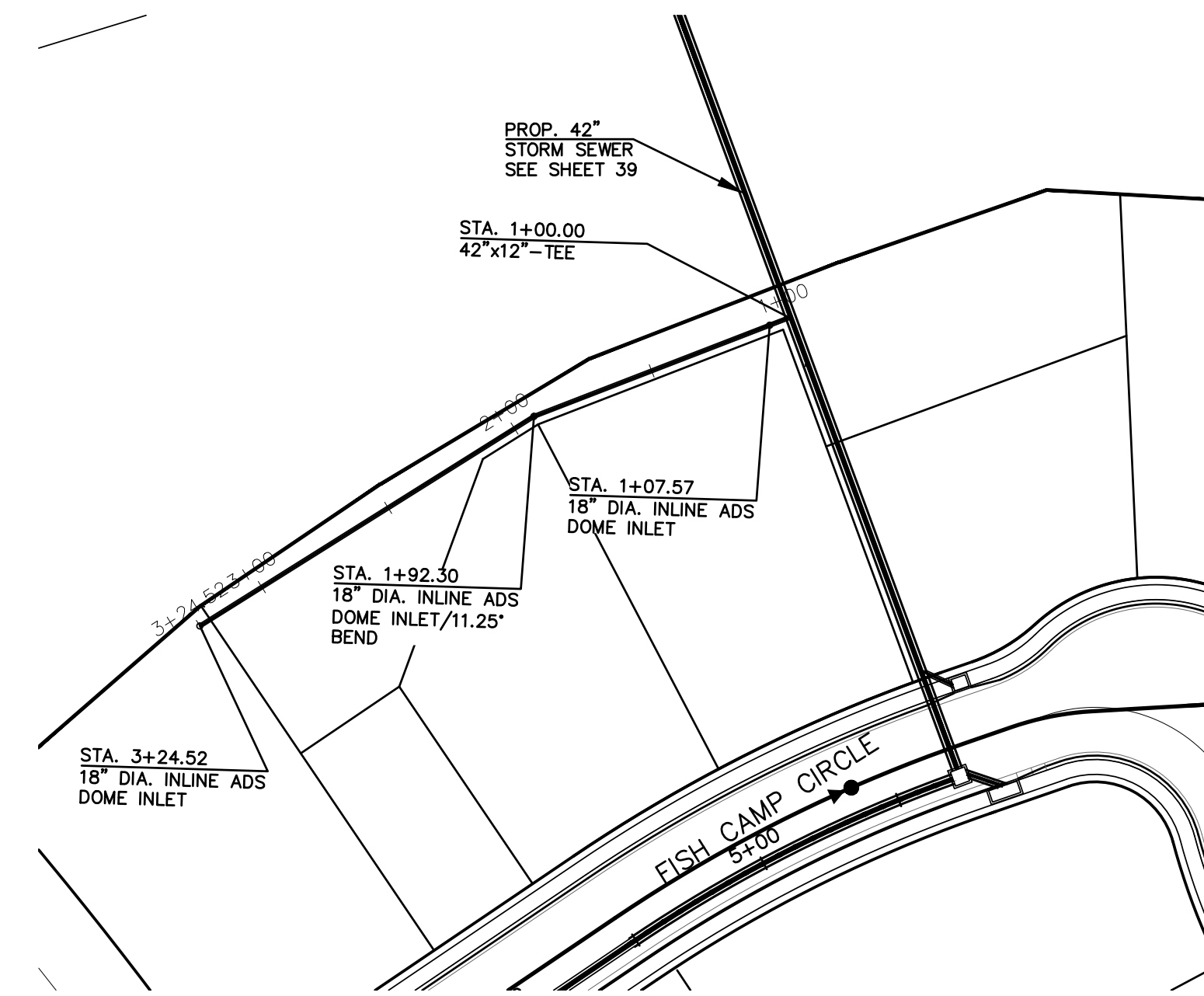
STORM SEWER LATERAL-14 (PIPE RUN 37) PROPOSED PRIVATE HDPE STORM SEWER 1" = 50' HORIZ. 1" = 5' VERT.
