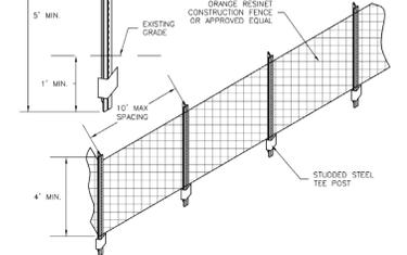
**CF-1. PLASTIC MESH CONSTRUCTION FENCE**
