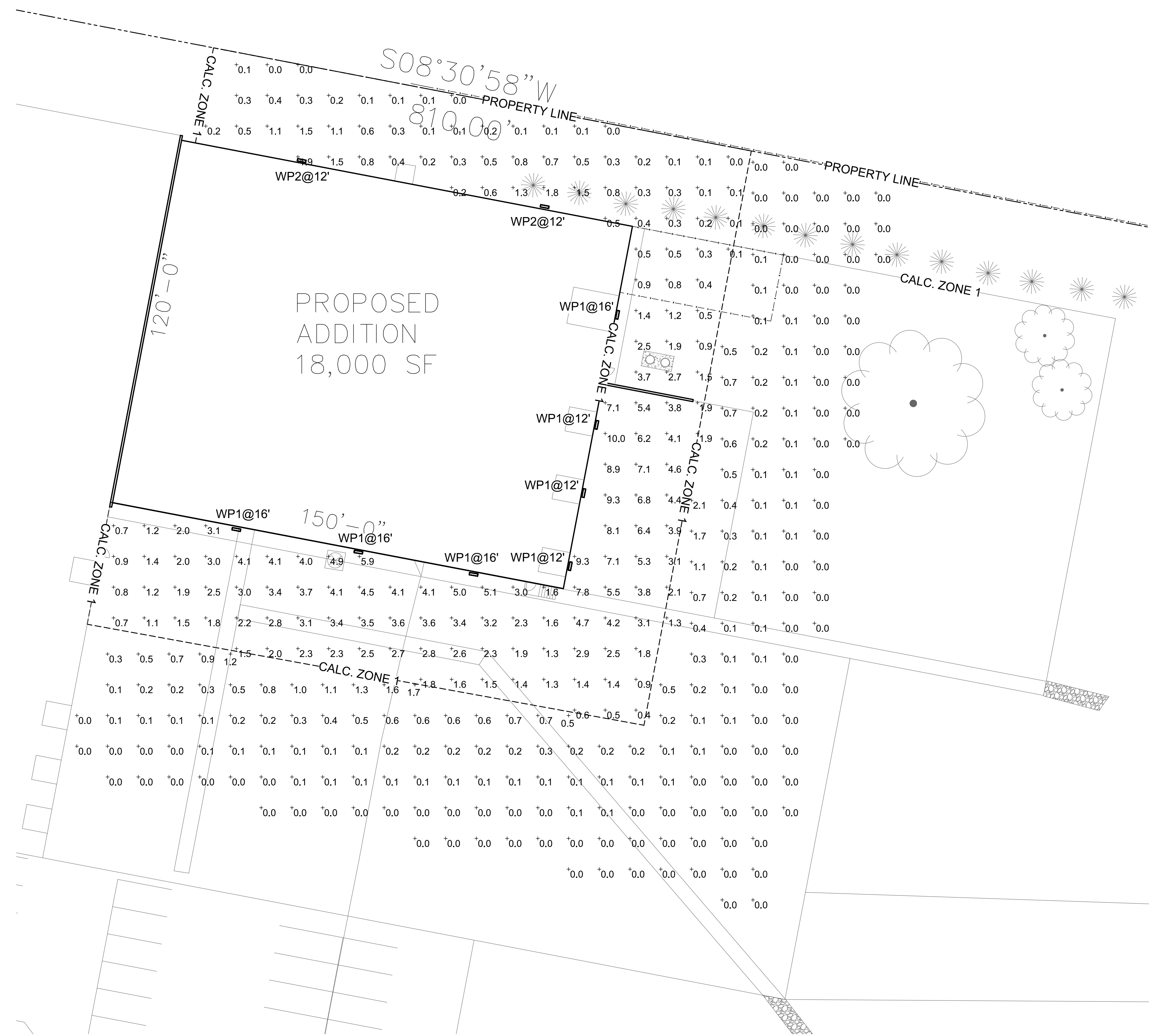
1 SITE PHOTOMETRIC PLAN ES1.1 SCALE: 1" = 30'-0"
