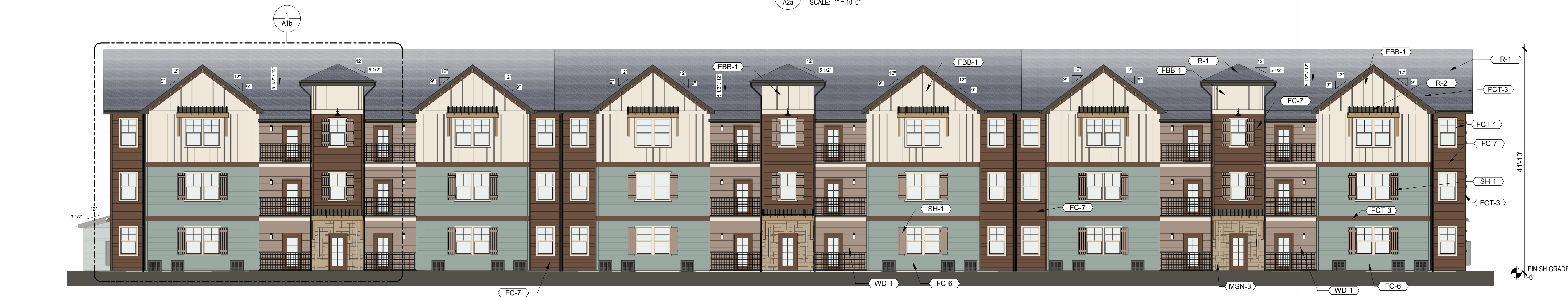
36 2B UNIT BUILDING - REAR ELEVATION SCALE: 1" = 10'-0"
