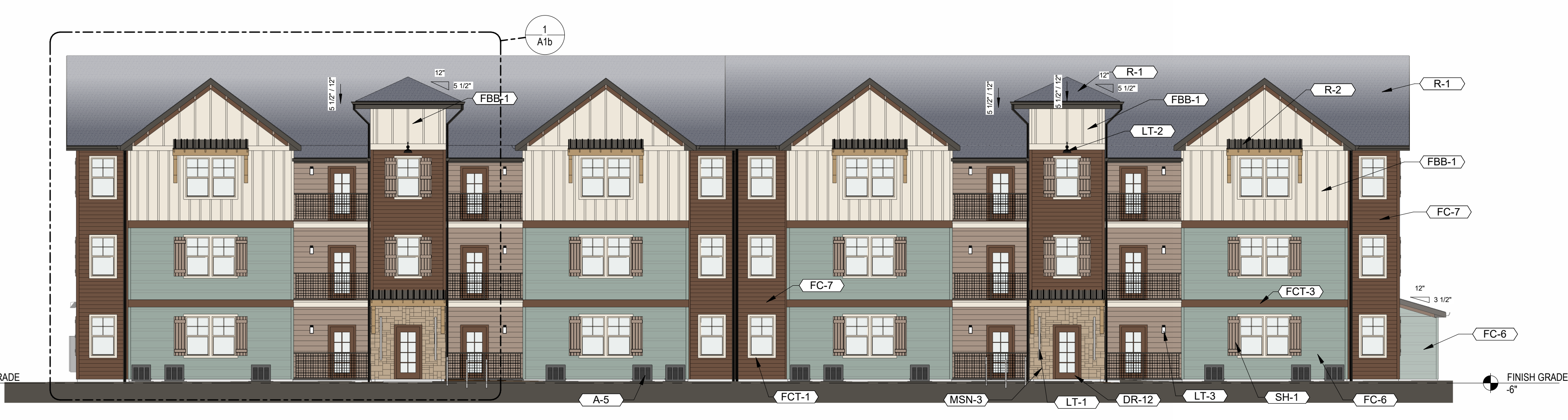
24 2B UNIT BUILDING - FRONT ELEVATION SCALE: 1" = 10'-0"
