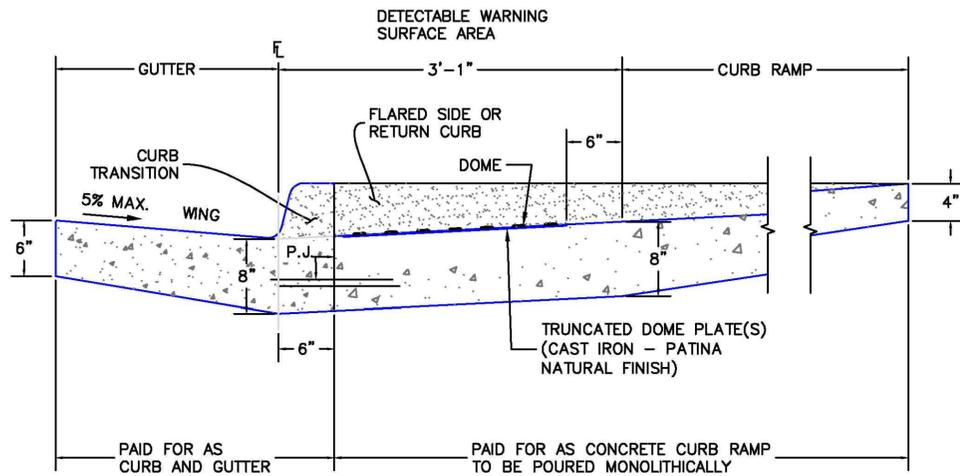
P.J. = PERMISSIBLE JOINT WITH EPOXY-COATED DEFORMED NO. 4 BARS CONFORMING TO AASHTO M 284 AT 18 IN. SPACING
