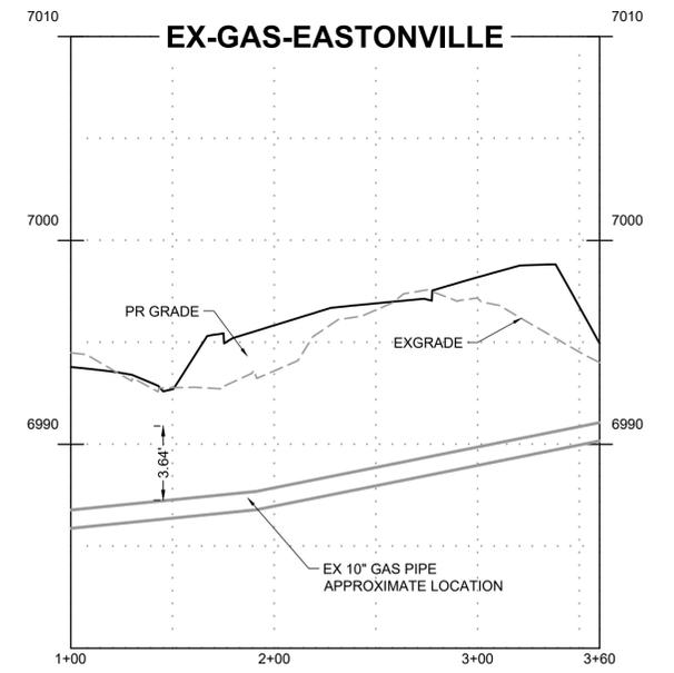
NOTE: CONTRACTOR TO VERIFY LOCATION AND ELEVATION OF GAS LINE PRIOR TO CONSTRUCTION
