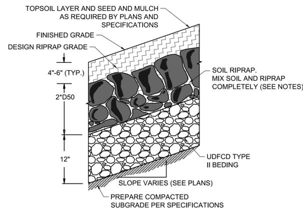
**SOIL RIPRAP EMBANKMENT PROTECTION
