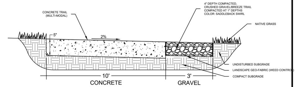
NOTE: REFER TO EL PASO COUNTY ENGINEERING CRITERIA MANUAL FOR CONCRETE SPECIFICATIONS AND DETAILS.
