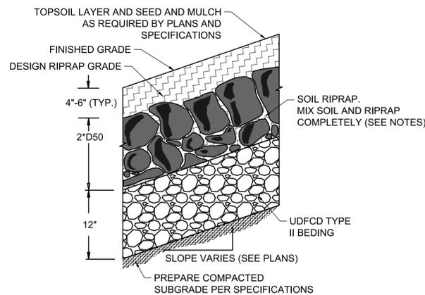
**SOIL RIPRAP EMBANKMENT PROTECTION
