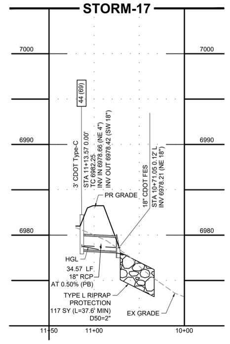
NOTE: ADD WATER TIGHT JOINT WHEN 100-YR HGL SHOWS PIPE FULLY INUNDATED.
