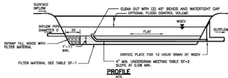
NOTE: THIS DETAIL SHOWS A PARTIAL INFILTRATION SECTION. FOR FULL INFILTRATION ELIMINATE UNDERDRAIN AND PROVIDE 1'-6" OF FILTER MATERIAL. FOR NO INFILTRATION PROVIDE IMPERMEABLE MEMBRANE SECURED TO CAST-IN-PLACE CONCRETE WALL. SEE DETAILS SF-2 AND SF-3.
