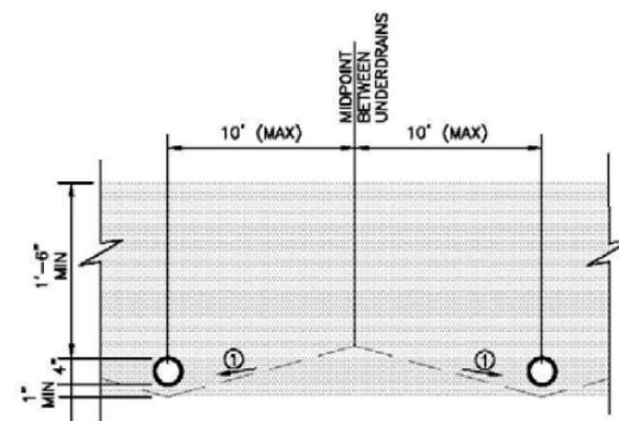
① SLOPE (STRAIGHT GRADE) SUBGRADE (2-10%) TO UNDERDRAIN TO REDUCE SATURATED SOIL CONDITIONS BETWEEN STORM EVENTS (OPTIONAL)
