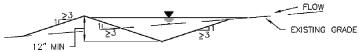
EARTH DIKE AND DRAINAGE SWALE INSTALLATION NOTES
