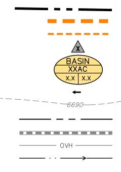
BASIN BOUNDARY-MINOR BASIN DESIGN POINT BASIN I.D. ACREAGE 5 YR/100 YR CFS DIRECTION OF FLOW EXISTING CONTOUR EXISTING ROW/LORSON RANCH BOUNDARY EXISTING STORM SEWER EXISTING OVERHEAD TRANSMISSION LINES
