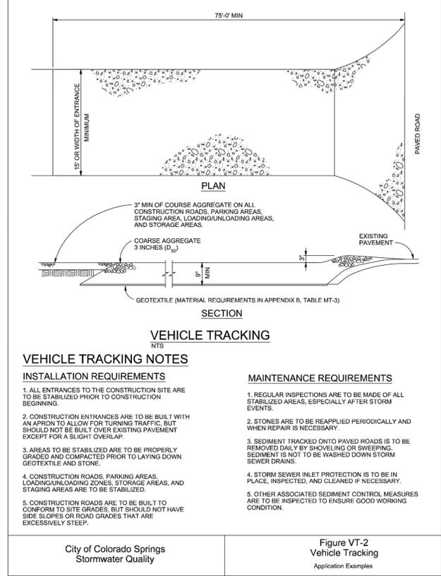
**Figure VT-2 Vehicle Tracking**
