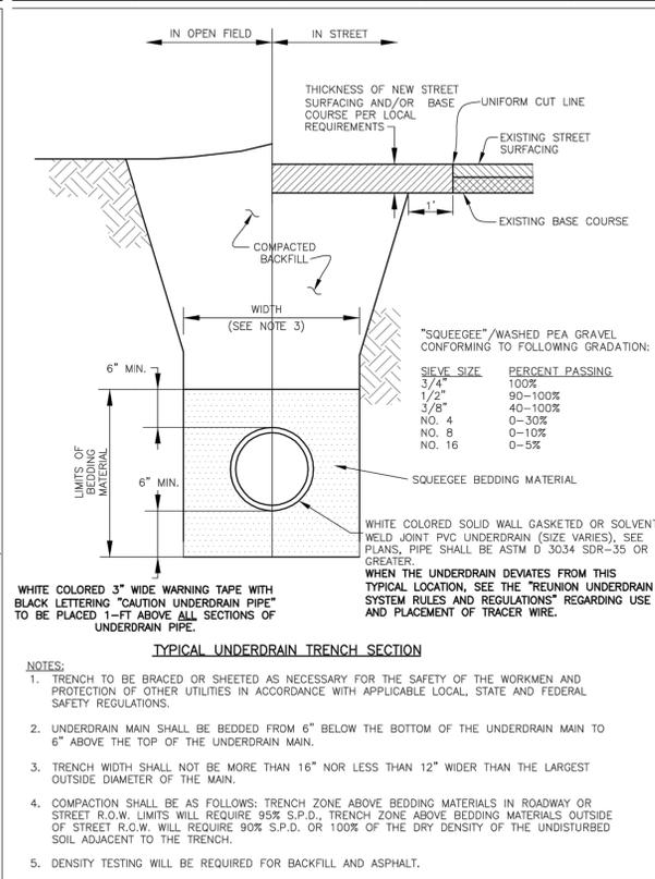
**UNDERDRAIN TYPICAL TRENCH OUTSIDE OF SANITARY SEWER**
