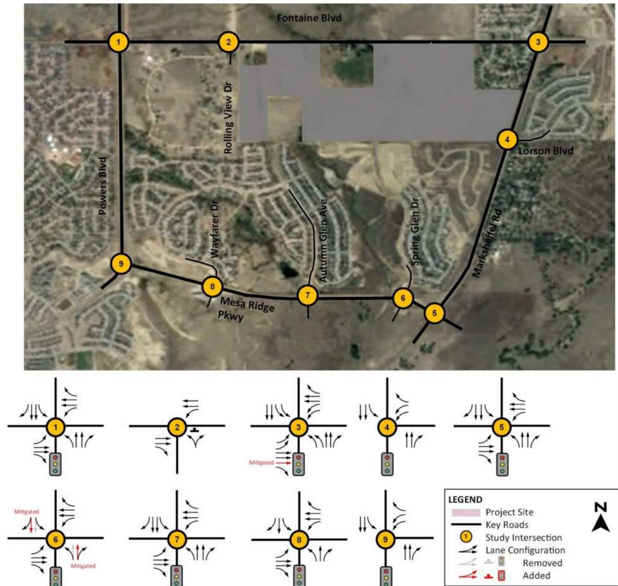
Figure 11 - 2040 Background Lane Configuration & Traffic Control
