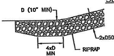
TERMINATION OF RIPRAP LINED SLOPE DRAIN
