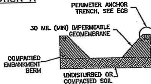
GEOMEMBRANE LINED SLOPE DRAIN
