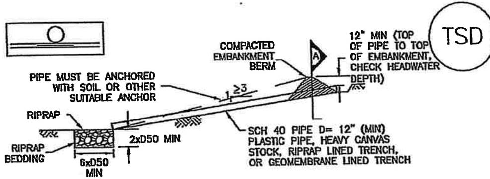
TEMPORARY SLOPE DRAIN PROFILE
