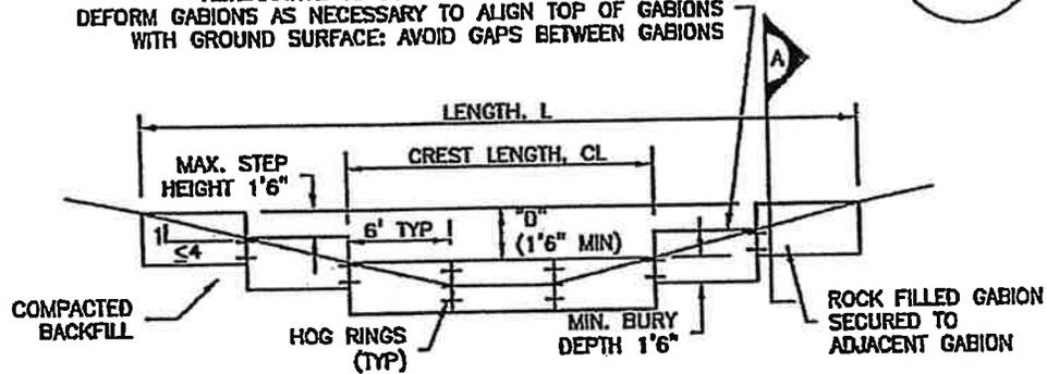
REINFORCED CHECK DAM ELEVATION VIEW
