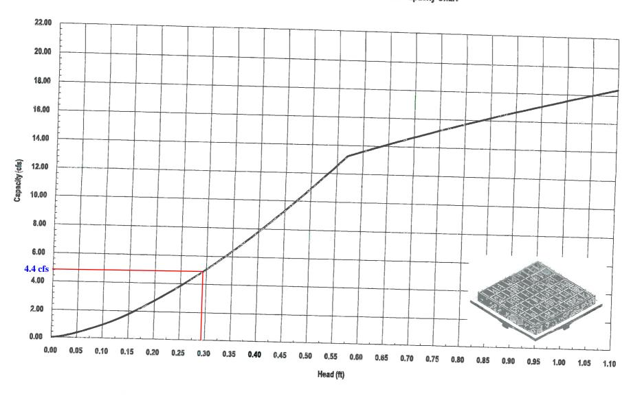
$DP10 = Q_{100} = 2.2 \text{ cfs } 50\% \text{ BLOCKAGE} = 4.4 \text{ cfs}$
