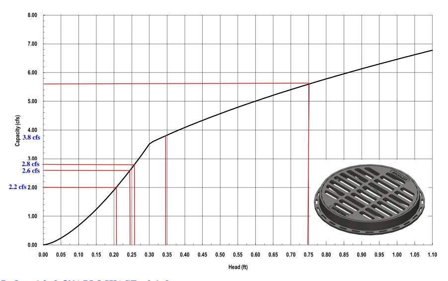
DP7= Q100=1.3 cfs 50% BLOCKAGE = 2.6 cfs DP9= Q100=2.8 cfs 50% BLOCKAGE = 5.6 cfs DP11=Q100=1.4 cfs 50% BLOCKAGE = 2.8 cfs DP12=Q100=1.0 cfs 50% BLOCKAGE = 2.0 cfs
