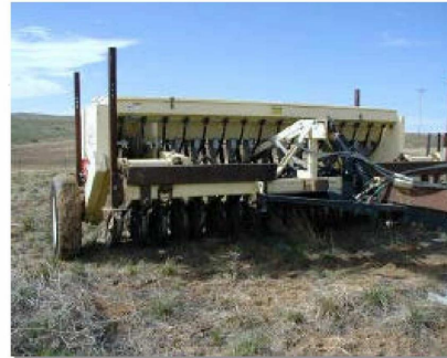
Photograph TS-PS-1: Equipment used to drill seed into soil. Photo courtesy of Douglas County.
