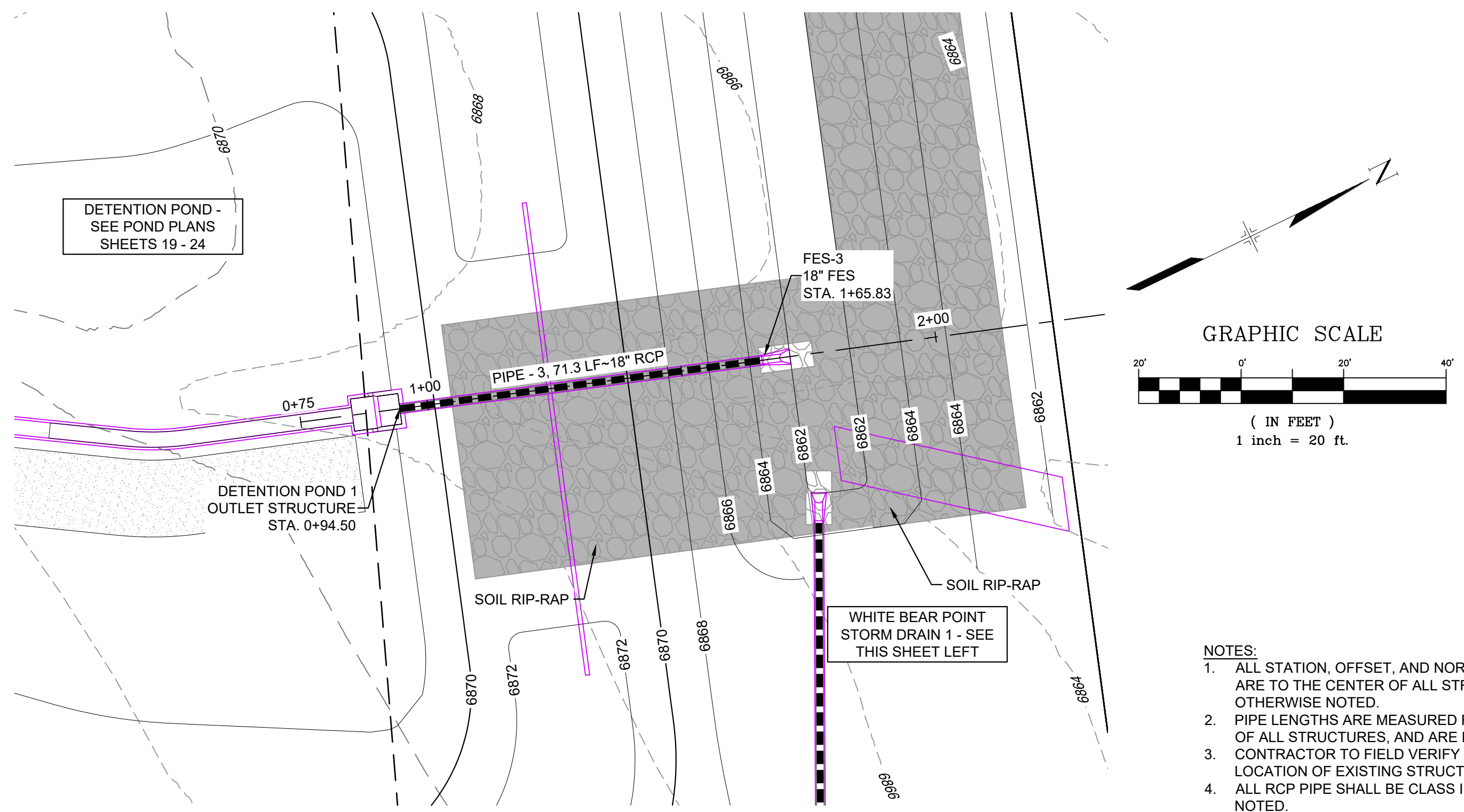
DETENTION POND OUTFALL STORM DRAIN PLAN
