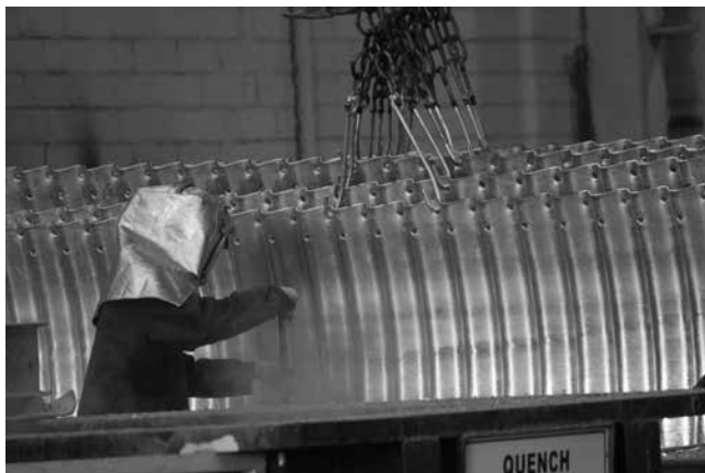
Hot-Dip Galvanizing Process
