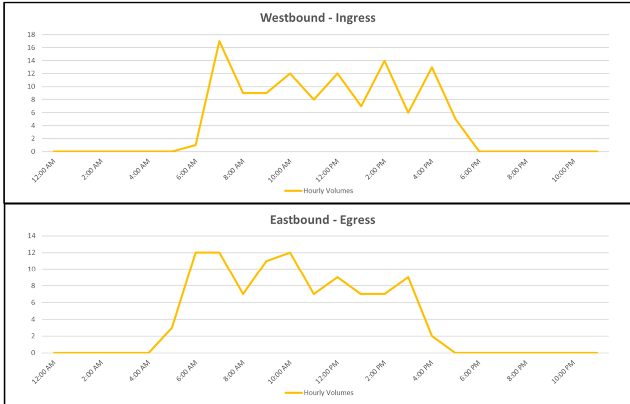
Figure 6: Site Driveway 24-Hour Volume Distribution
