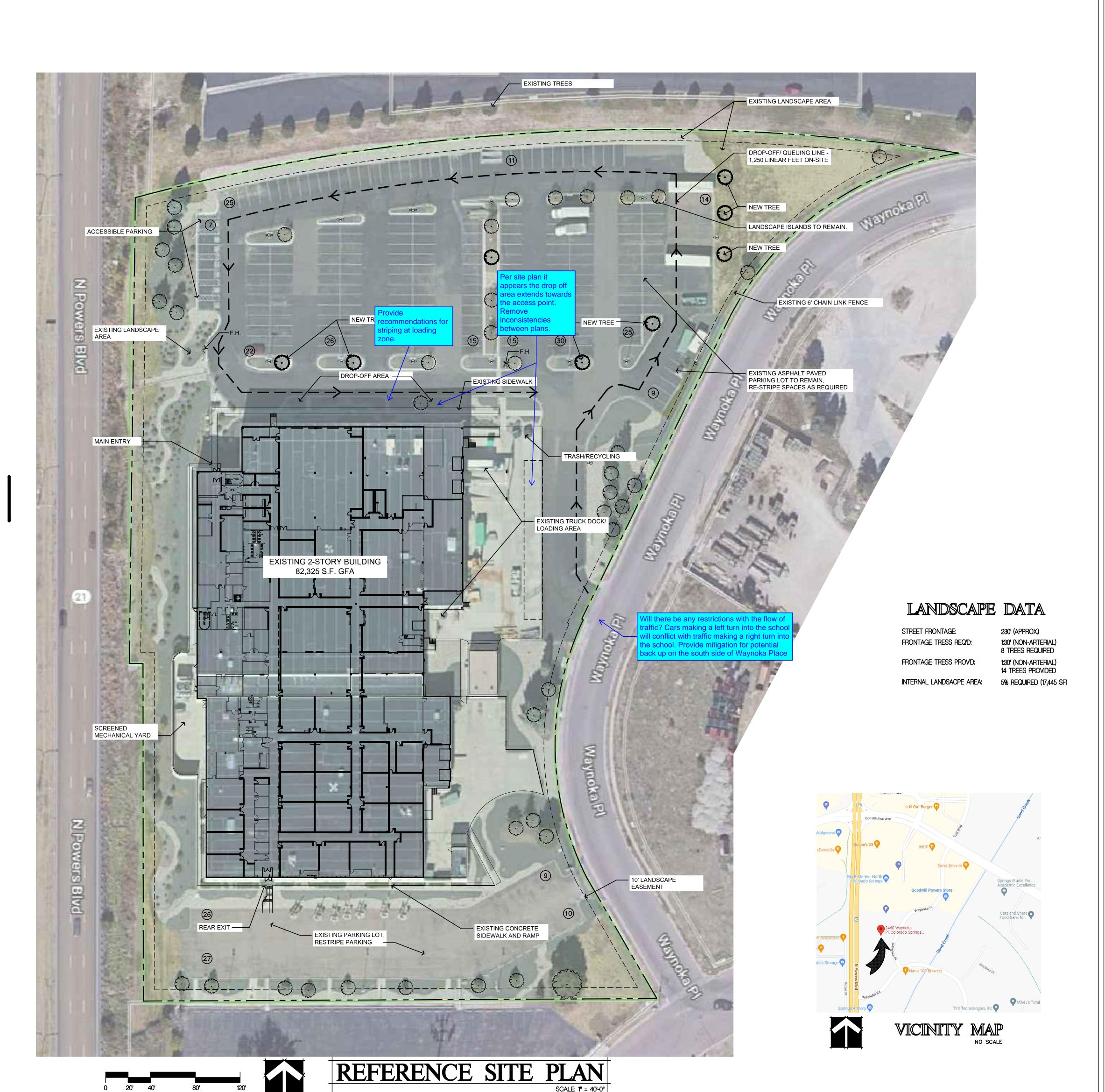
PROJECT DATA P-TEC INTERIOR REMODEL CHANGE OF USE PROJECT DESCRIPTION: INTERIOR REMODEL OF AN EXISTING FABRICATION FACILITY FOR A NEW CHARTER HIGH SCHOOL, INCLUDING VOCATIONAL TRAINING AREAS. SITE WORK LIMITED TO ACCESSIBLE ACCESS UPGRADES.
