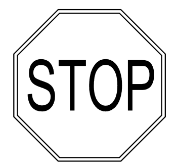
30"x30" MINIMUM SIZE BACKGROUND 4090 (3M-WHITE DIAMOND GRADE) OR EQUIVALENT 1172 C (3M-RED EC FILM) OR EQUIVALENT MUTCD R1-1 STOP SIGN DETAIL NOT TO SCALE
