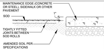
**A SOD INSTALLATION NOT TO SCALE**
