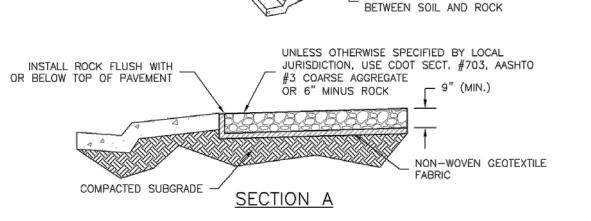
VTC-1. AGGREGATE VEHICLE TRACKING CONTROL
