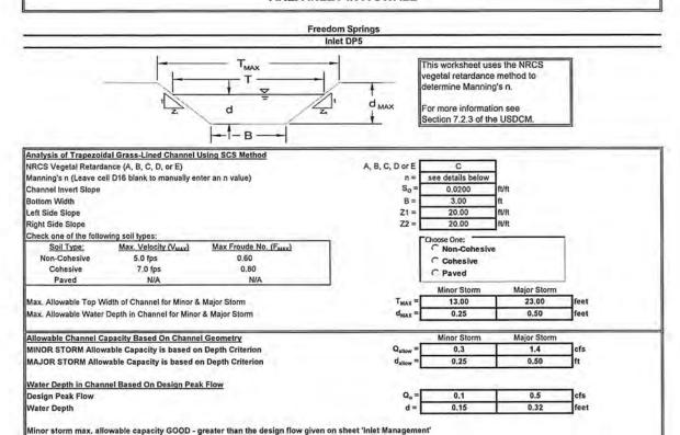
Major storm max, allowable capacity GOOD - greater than the design flow given on sheet 'Inlet Management'
