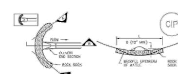
CIP-1, CULVERT INLET PROTECTION
