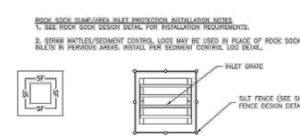
IP-4, SILT FENCE FOR SUMP INLET PROTECTION
