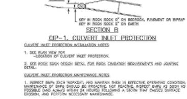
CIP-1, CULVERT INLET PROTECTION
