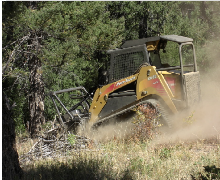
Machine mastication with skid steer
