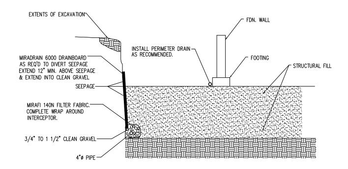
NOTE: EXTEND INTERCEPTOR DRAIN TO UNDERDRAIN OR TO SUMP. BENCH DRAIN INTO NATIVE SOILS 12 INCHES MINIMUM.
