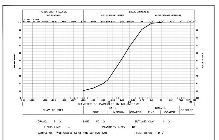
These test results apply only to the samples which were tested. The testing report shall not be reproduced, except in full, without the written approval of Kumar & Associates, Inc. Sieve analysis testing is performed in accordance with ASTM D6913, ASTM D7928, ASTM C136 and/or ASTM D1140.
