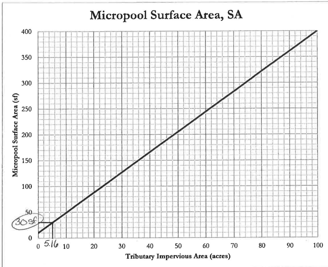
**Figure 1 – Micropool surface area (SA) determination chart**
