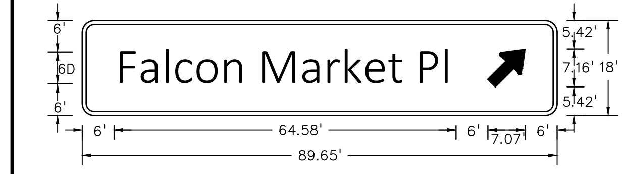
D1-1d CIRCULAR INTERSECTION EXIT DESTINATION (1 LINE) 2.25" RADIUS, 0.75" BORDER, WHITE ON GREEN [Falcon Market Pl] 6D
