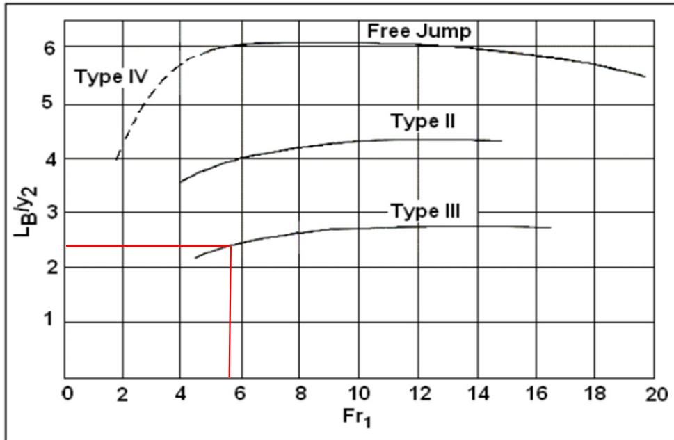
Figure 8.2. Length of Hydraulic Jump on a Horizontal Floor
