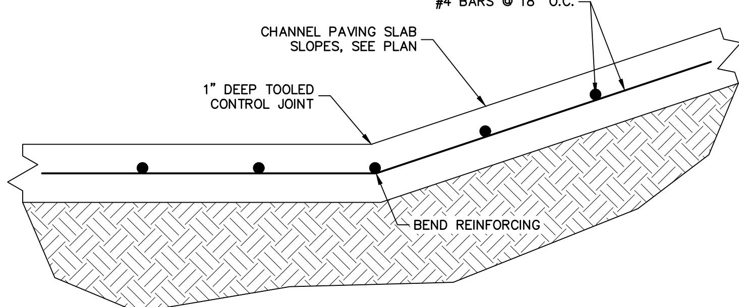
SLOPE CHANGE AT CHANNEL PAVING SLAB
