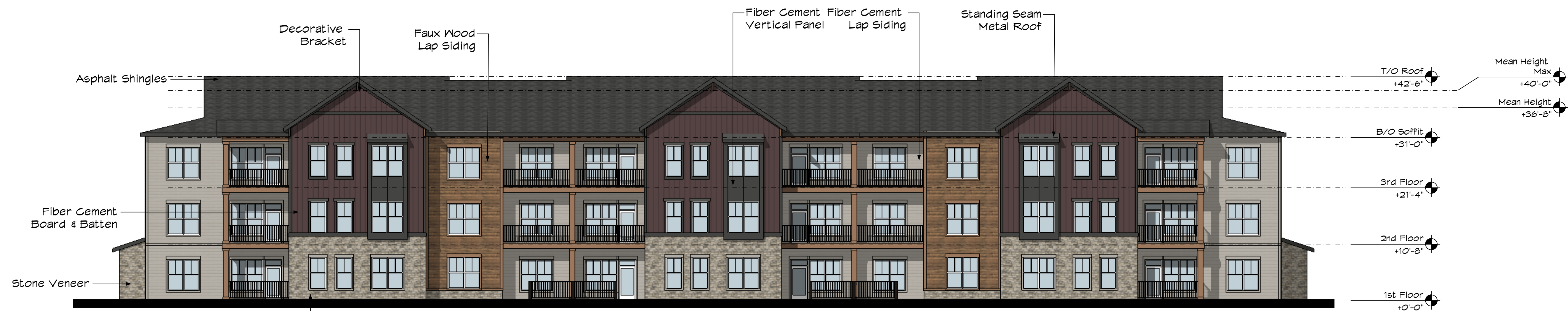
BACK ELEVATION - BUILDING TYPE C Scale: 3/32" = 1'-0"
