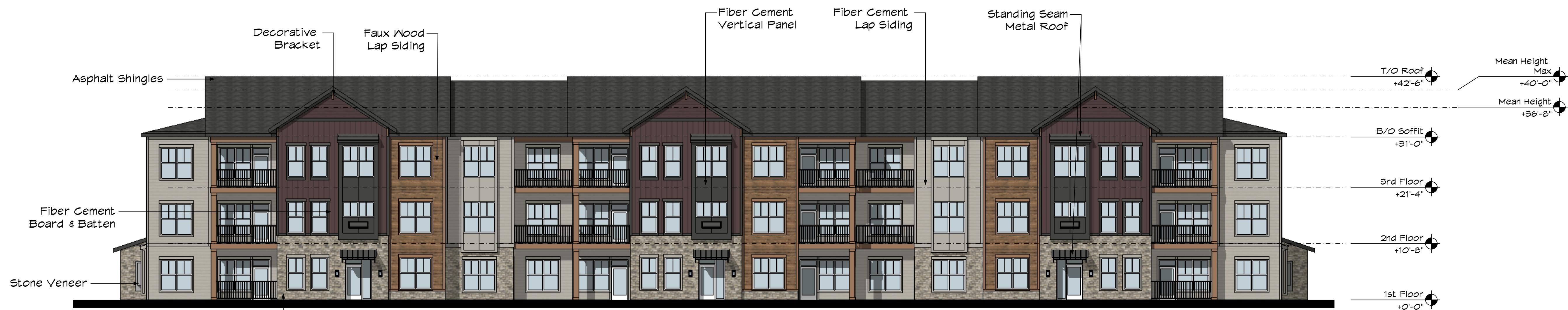
FRONT ELEVATION - BUILDING TYPE C Scale: 3/32" = 1'-0"
