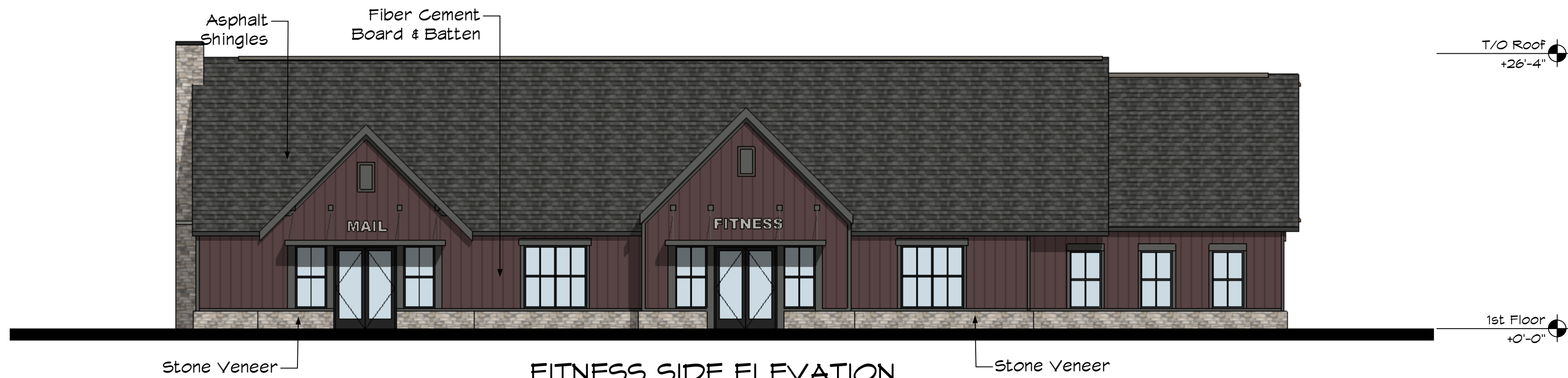
FITNESS SIDE ELEVATION Scale: 1/8" = 1'-0"
