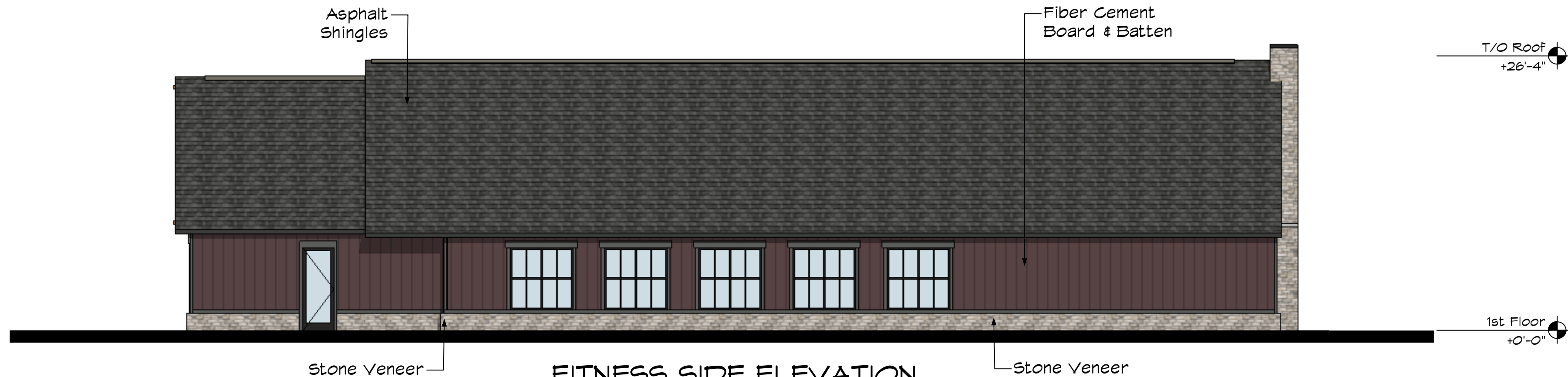
FITNESS SIDE ELEVATION Scale: 1/8" = 1'-0"
