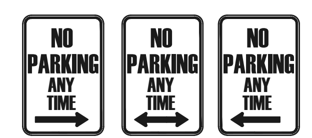
NO PARKING SIGN (R7-1)
