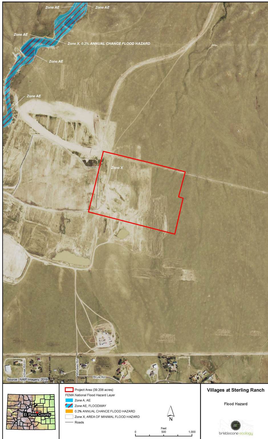
Figure 7: Flood Hazard Map
