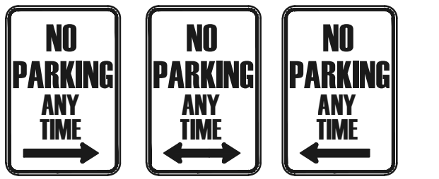
NO PARKING SIGN (R7-1)
