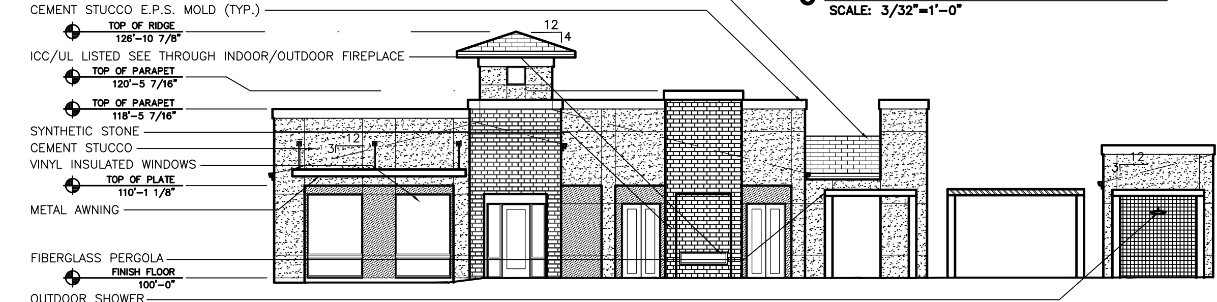
7 NORTH CLUBHOUSE & EQUIPMENT BUILDING ELEVATIONS SCALE: 3/32"=1'-0"
